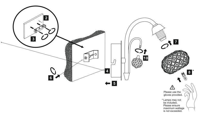
Voltage: 230V - 50/60Hz Lampholder: G9 Lamps: 1 x 33W Max
